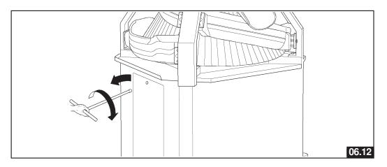
■ Loose the tension rod 07.12 (01) by using wrenches.07.12 (01)
